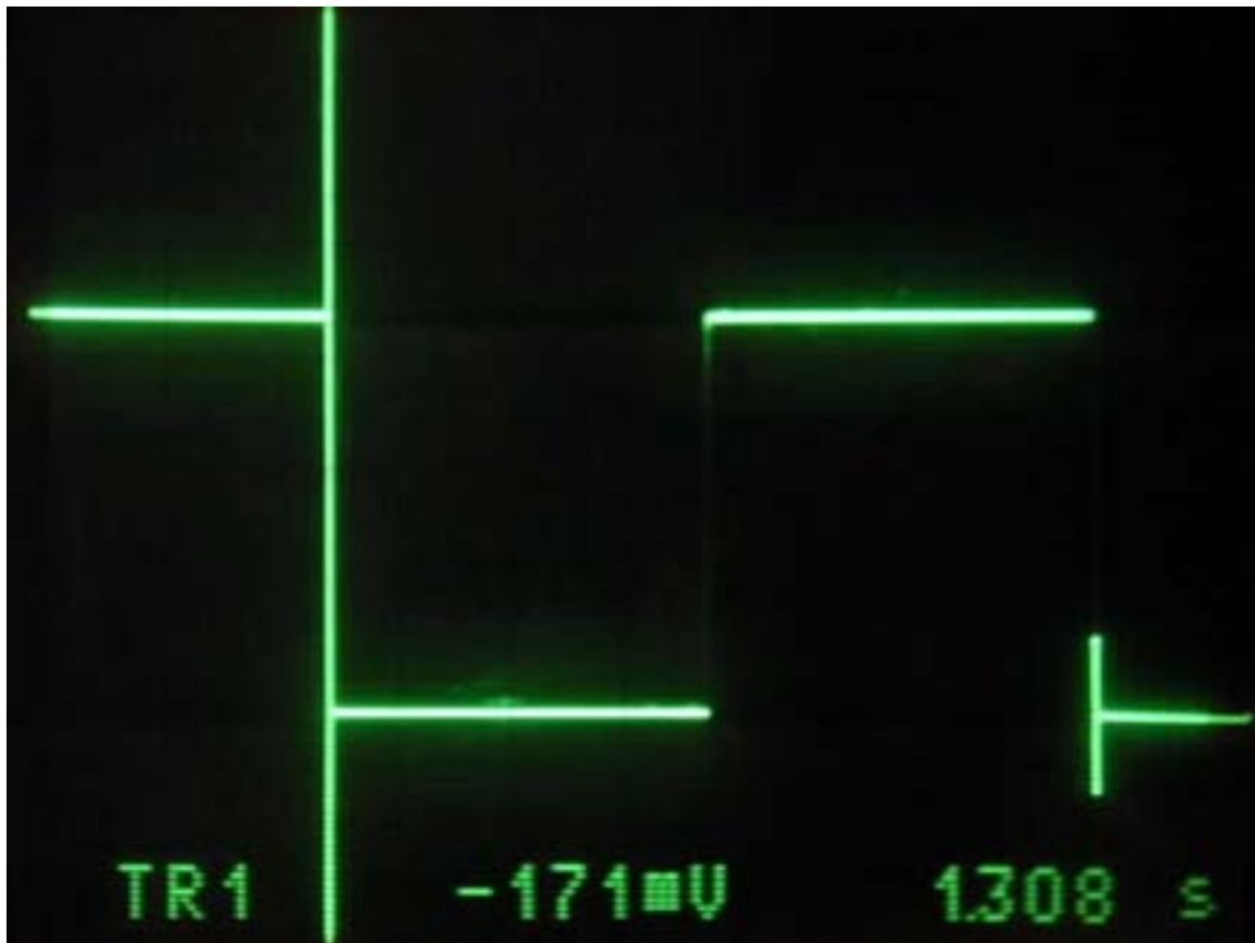
Figure 3. Comparator output; horizontal scale = 200mS/div, vertical scale = 500mV/div, supply voltage = 1.7V, amplitude = 1.7Vp-p, period = 1.308 seconds.
